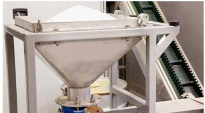
Hopper loaded with metal grain
